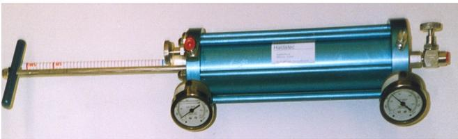
introducing a pressure gas source to the underside of the piston. This will enable the introduction of the sample or product to an analyser or pressurised pipeline.
