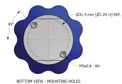
41 mm [1.61 in] A/F PT-C-024-001 (STAINLESS STEEL) PANEL MOUNT RING
