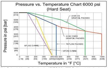
Note: Body material specifications based on ASME B16.34 - 2009. Packing material ratings based on manufacturer's specifications. Approximations only. Phoenix does not represent these values as finite. They are provided only as representative values.
