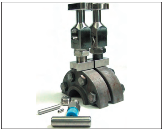
Step 3: Remove 1st bonnet plug
