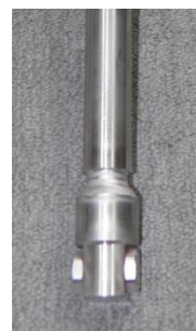
Quill with replaceable infusion spray nozzle
